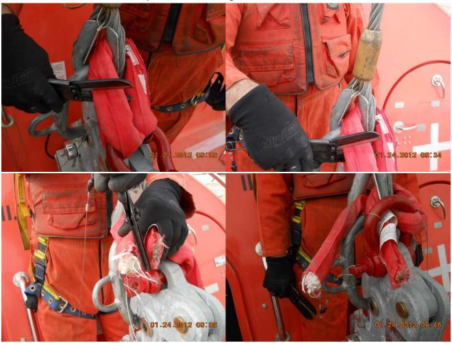
Note if the lifeboat has drifted away from the rig the fall wire will swing to a position directly under the launching station. Please anticipate the swing of the cable and know that it may not be completely predictable controllable by the person cutting the FPD. PLEASE THINK AHEAD
